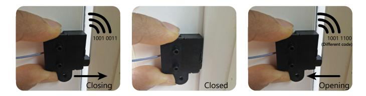
A ZF micro-generator powering a custom RF transmitter packaged as the Airy Sensor (black) shown here monitoring a swing door operation. When the door is opened or closed, the sensor sends a unique code (*without needing any battery*) to our WiFi hub, which relays it to the user through an App.
