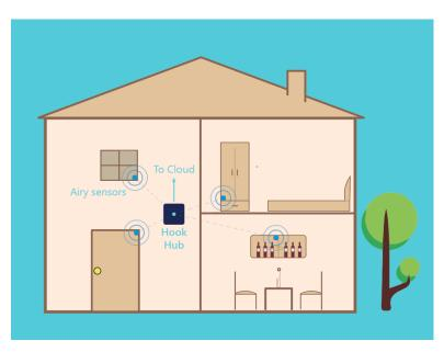
Airy sensors can be installed to monitor **doors** (single, double and sliding), **windows** (horizontal and vertical), and **closets** and **cabinets** (liquor, jeweler etc.) for operation. The sensors send the signal wirelessly to the central Hub. The Hub relays the commands to the cloud which sends it to the user's Smartphone.
