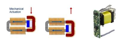
(left) Mechanical actuation moves a permanent magnet which results in change in magnetic flux in the coils thus creating electric impulse. The electric impulse powers a RF radio that transmits a coded message (ZF AFIM 5002, right). Another message is sent when the spring-loaded magnet retracts. Images from zf.com.
