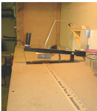
Gary the Chopper. Rigged up hot knife for cutting different webbing lengths. Out of the box it is a manual cutter. After some modifications it is now operated with a foot pedal.
