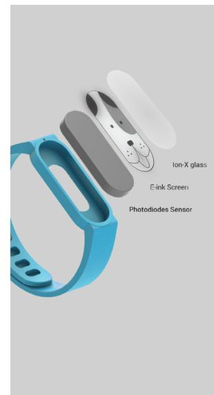
Aibi is a three part system that offers early detection, treatment instruction, and communication between patients and their caretakers. The Aibi system consists of a wearable bracelet that tracks histamine levels on the skin, a redesigned medicine applicator, and a communication system that works over the cellphone emergency alert system.
